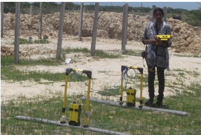
Figure 8: GPR profiling and groundwater analysis in the field
