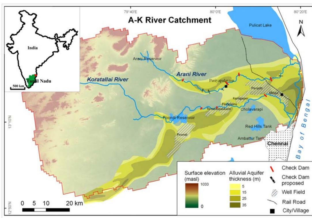
Figure 4. Topography and aquifer thickness of the Arani–Koratallai river catchment near Chennai. Extent and thickness of alluvial aquifer and well field location from Charalambous and Garratt (2009), digital surface model from SRTM data, A–K river catchment from Hydro1 K (USGS 2008) (Sprenger et al. 2014).
