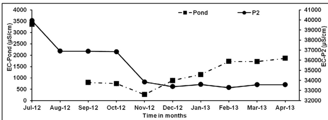
Figure 15. Temporal variation in electrical conductivity of water in the pond water and piezometer (Raicy and Elango, 2014b).
