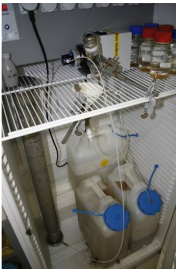
Figure 7-2 Column-apparatus to determine the breakthrough of coliforms under laboratory conditions (Sandhu et al. 2013)
