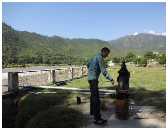
Figure 5-2 Pumping test and sampling being conducted on MW5 and PW5, Srinagar (Photo: V. Nguyen, HTWD, 2012)
