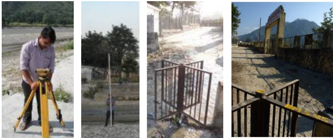
Figure 5-3 (from left to right) Levelling instrument (dumpy level), staff and the revolving door used as a datum (benchmark) for surface water level measurements
