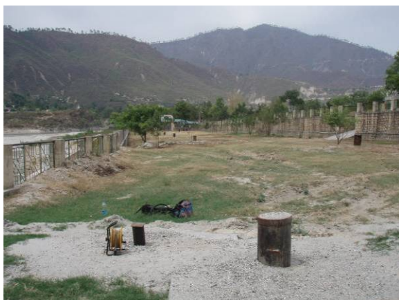
Figure 5-1 Monitoring well MW5 (left) constructed in between PW5 (right) and Alaknanda, Srinagar (Photo: HTWD, 2012)
