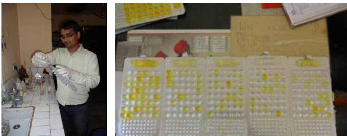
Figure 5-7 Preparation of water samples and enumeration of coliform counts using the IDEXX Colilert-18 method (HTWD and UJS 2013)
